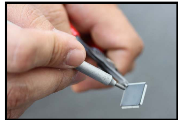
Microblasting can be used to alter component surfaces
