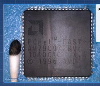
Remarking & Resurfacing Testing Revealed: Parts Failed Resistance To Solvents (RTS) -Acetone
