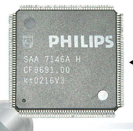
External markings test/inspection
