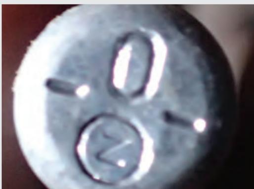
**An electric detonator produced in the Czech Republic**
