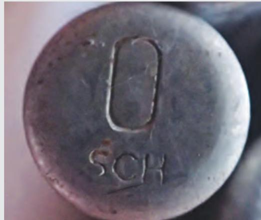
**An electric detonator produced in Austria**
