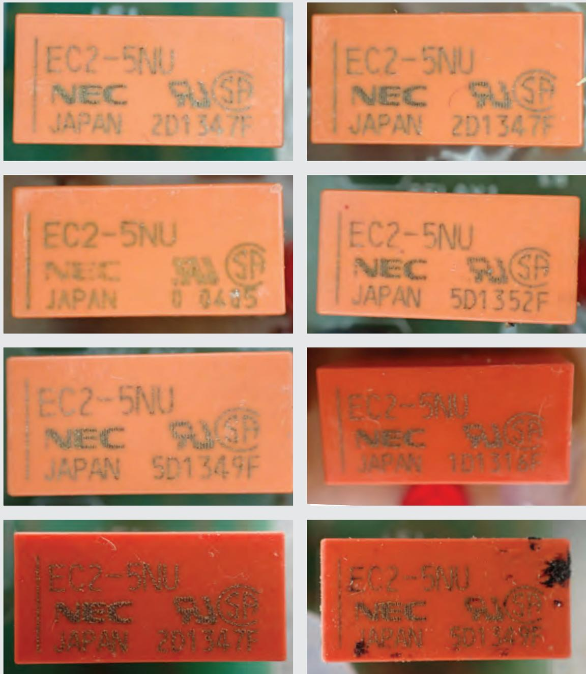
**EC2 signal relays produced by NEC TOKIN**
