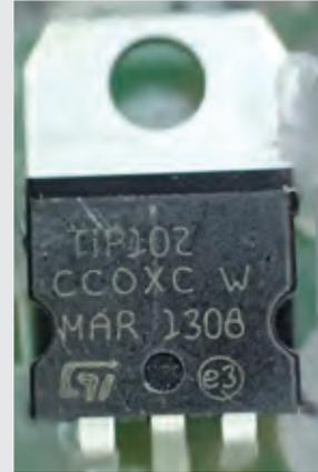
**A TIP102 transistor produced by STMicroelectronics**
