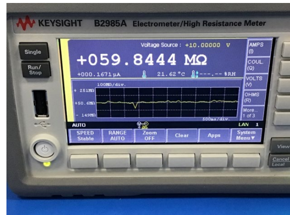
Fig 18 Insulation resistance measurement of a qualified MLCC using the B2987A Electrometer/High Resistance Meter.
