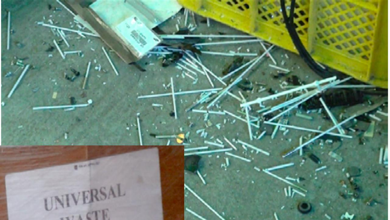
**Figure 42. (above)** CCFL tubes, which contain toxic mercury phosphors. ©BAN. December 2015.
