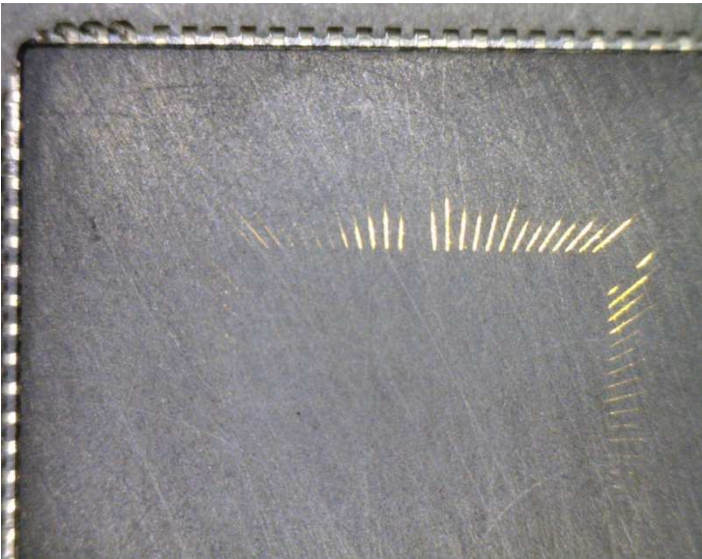
Figure 5: External view of sample after over-sanding
