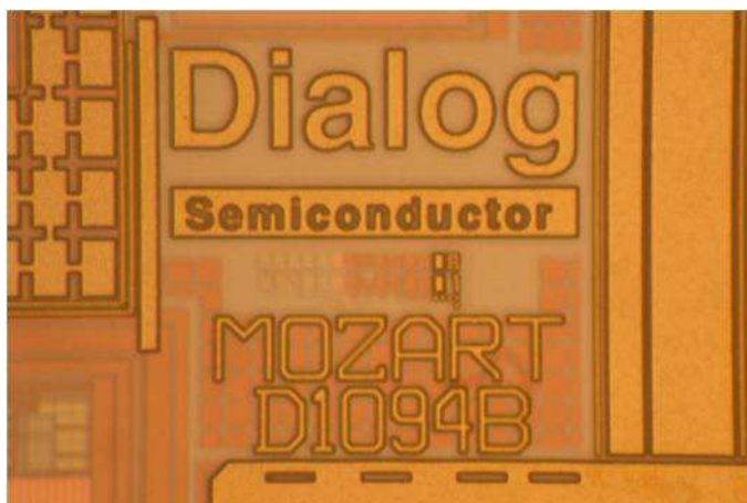
Figure 1: Displays die level markings of Dialog Semiconductor Mozart D109B
