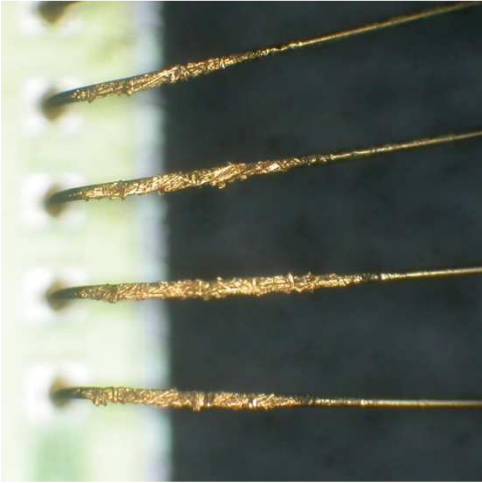
Figure 4: Result of over-sanding to remove original external markings
