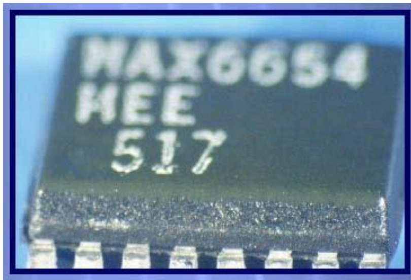
Counterfeit Unit Showing Non Uniform Black Coat Layer
