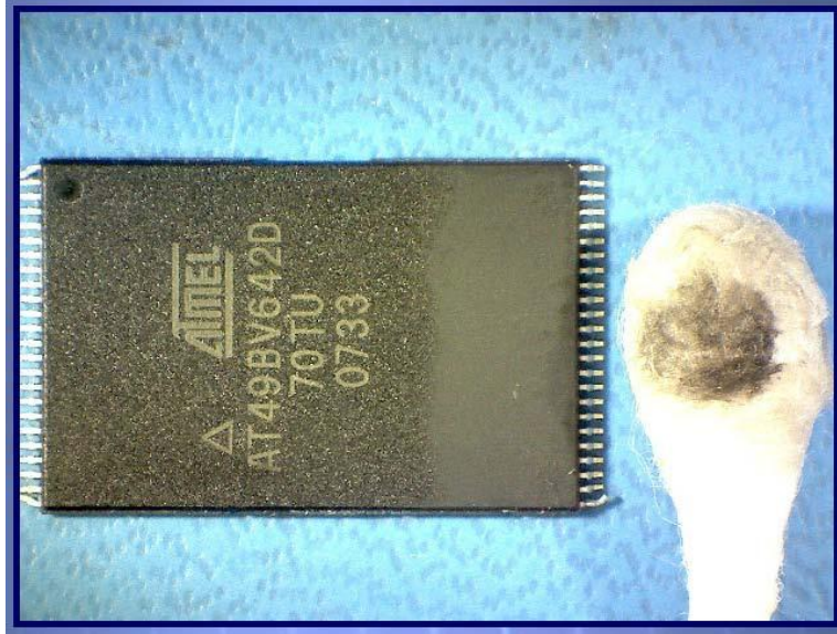
Part Failing Acetone Test
