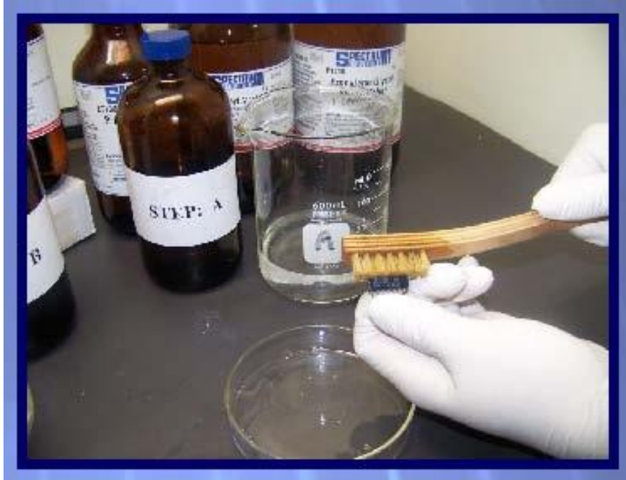
Application of Resistance to Solvents Test Marking Permanency Per MIL STD 883, Method 2015.3 Step A
