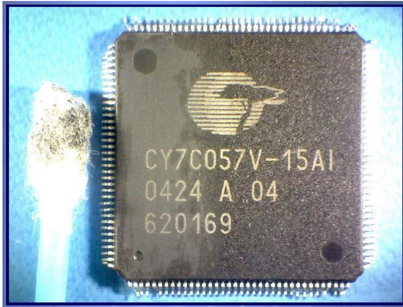
Part Failing Dynasolve Test
