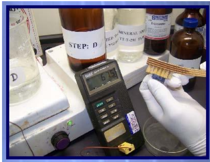
Application of Resistance to Solvents Test Marking Permanency Per MIL STD 883, Method 2015.3 Step D, including chemical heating
