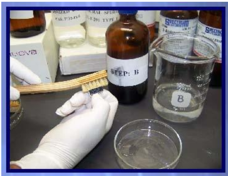
Application of Resistance to Solvents Test Marking Permanency Per MIL STD 883, Method 2015.3 Step B
