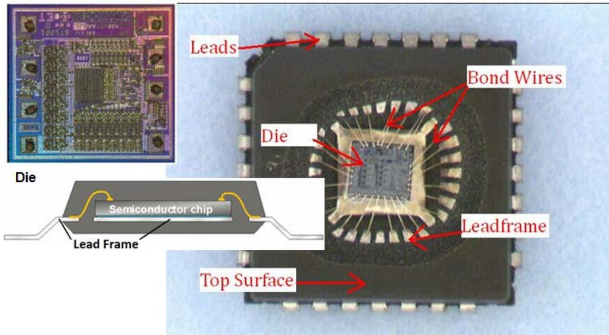
**Figure 6: Overview of Integrated Circuit**
