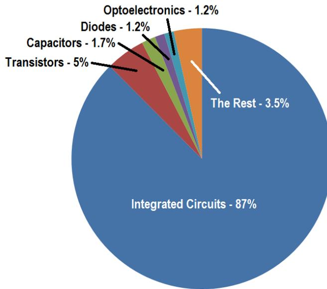
Figure 2: Breakdown of Counterfeit Electronic Parts
