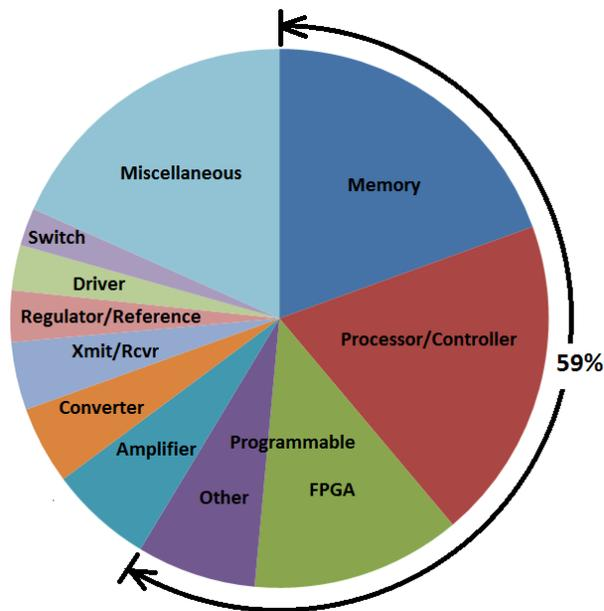
Figure 3: Breakdown of Counterfeit Integrated Circuits
