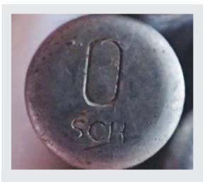
An electric detonator produced in Austria
