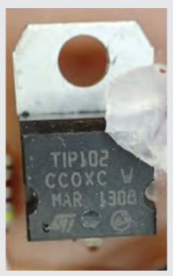
**TIP102 transistors produced by STMicroelectornics**
