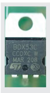
A BDX53C transistor produced by STMicroelectronics
